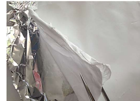
electrospun on an aluminum foil
