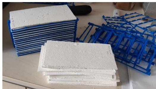
Adsorbent layer stack preparation
